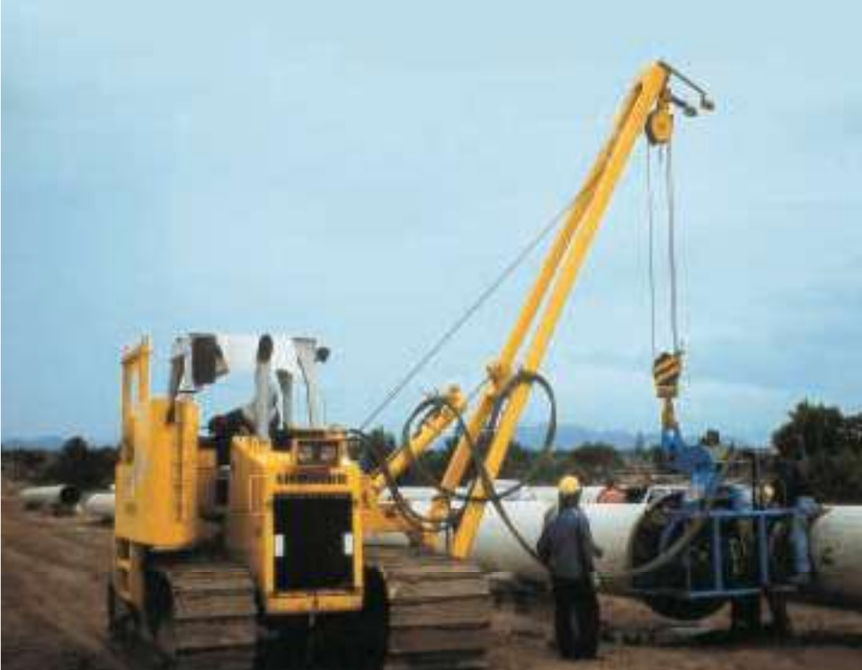
Pipefacing. The hydrostatic travel drive and the single joystick control allows exact placement of pipes.
